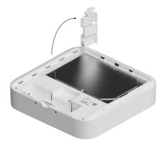
**4.** Install the hard drive in the NVR enclosure so that the connectors match.
