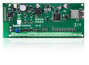
The system can be configured in two ways: from a computer with PERFECTA Soft program installed (locally – connection via RS–232 (TTL) port, remotely – using data transmission over Ethernet), as well as from a keypad, using key sequences in the service menu.
